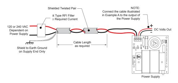
Figure 2.2.5: AC Cabling - 50 Feet or Greater - AC To Power Supply
